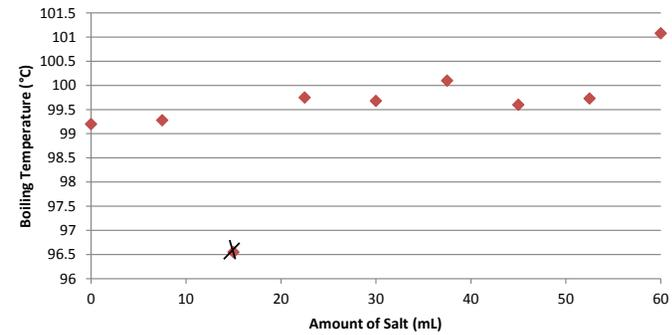
When relating the amount of salt to boiling temperature, the general trend is that an increase in the amount of salt leads to an increase in the boiling temperature. The control with no salt boils at 99.2°C, while the sample containing 60 ml of salt boils at 101.8°C, a total boiling temperature increase of 2.6°C. The sample with 15 ml of salt showed an unusual drop in temperature to 96.55°C, and has therefore been neglected; this can be attributed to experimental error.
