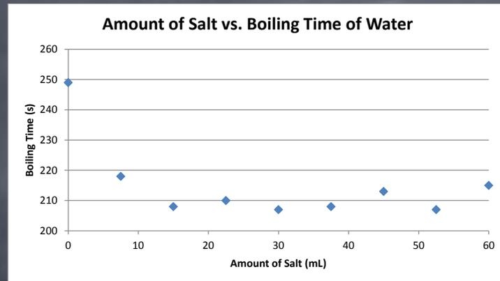
From this graph relating the amount of salt in the sample to the time it takes to boil, it can be seen that from the control (the sample containing no salt) to the first addition of salt, there is a significant drop in the time it takes to boil. The control took 249 seconds to boil while the sample with 7.5 ml of salt takes 218 seconds, a drop of 31 seconds. From there, the graph also shows that the amount of time remains in the 218 range, and does not go above the initial drop.
