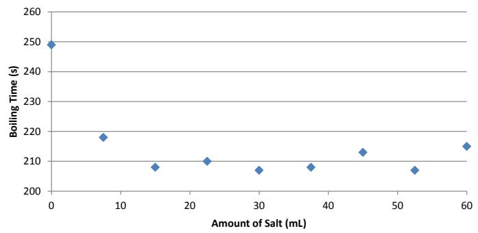
From this graph relating the amount of salt in the sample to the time it takes to boil, it can be seen that from the control (the sample containing no salt) to the first addition of salt, there is a significant drop in the time it takes to boil. The control took 249 seconds to boil while the sample with 7.5 mL of salt takes 218 seconds, a drop of 31 seconds. From there, the graph also shows that the amount of time remains in the 218 range, and does not go above the initial drop.
