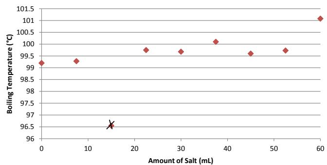
When relating the amount of salt to boiling temperature, the general trend is that an increase in the amount of salt leads to an increase in the boiling temperature. The control with no salt boils at 99.2°C, while the sample containing 60 mL of salt boils at 101.2°C, a total boiling temperature increase of 2.6°C. The sample with 15 mL of salt showed an unusual drop in temperature to 96.55°C, and has therefore been neglected; this can be attributed to experimental error.
